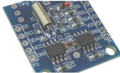
Raspberry Pi RTC Modul steuern - I2C Real Time Clock
